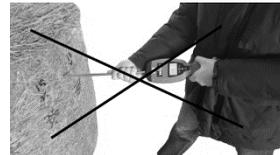
When measuring a bale with thick wrapping, puncture the wrapping with the probe tip before measurement to make sure the force required for making a hole in the wrapping will not affect density measurement.
